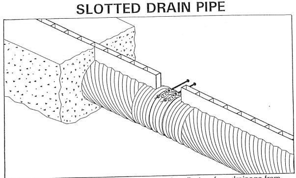
**Slotted Drain Pipe** is designed to effectively collect surface drainage from flat slope areas, sage inlets, or curb and gutter installations.
